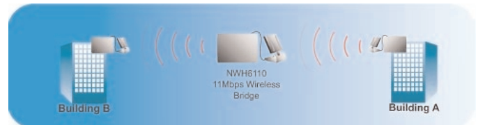
(right) Repeater Mode: Use the bridge as a repeater to extend the coverage range or to overcome an obstacle that blocks radio communication.
